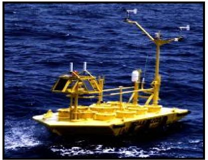
6-meter NOMAD Buoy 2, 215 nm S-SE Hilo (Courtesy NWS National Data Buoy Center)
