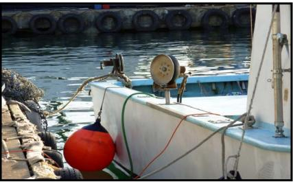
Offshore Handline Vessel with Hydraulic Line Puller, Kewalo Basin, 2006
